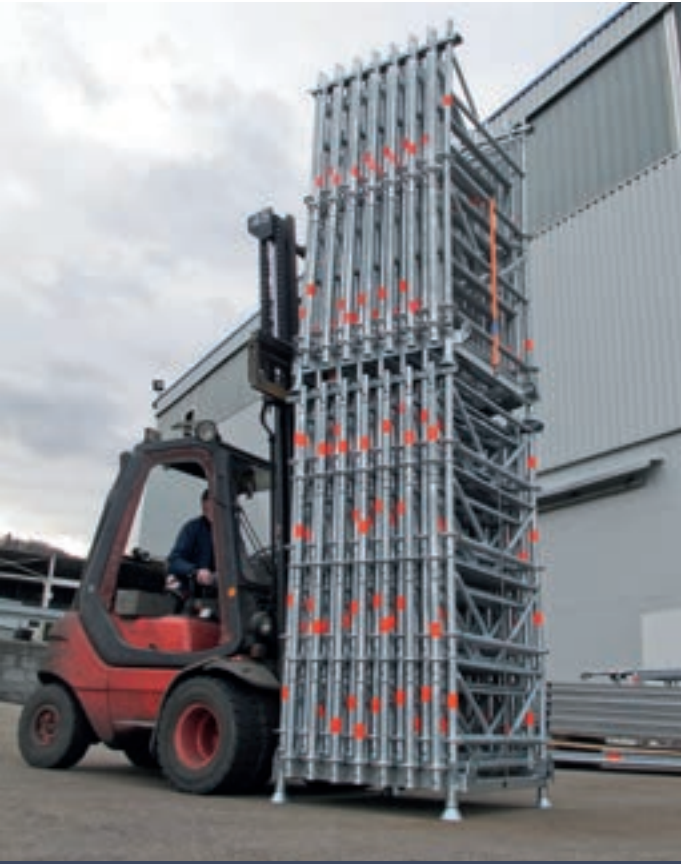
Filled and stacked TG 60 frame pallets for transport using a fork-lift truck
